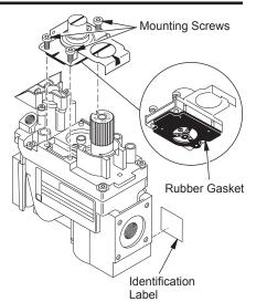
Figure 6 - Installing Pressure Regulator Assembly
